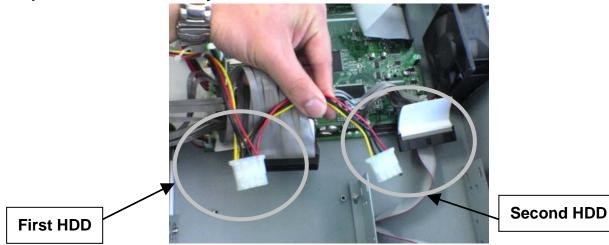
Figure 7: Wiring the two sets of HDD's
